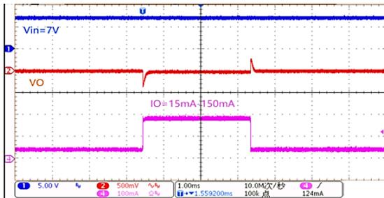
$V_{IN} = 7V, C_{IN} = 1\mu F, C_{OUT} = 1\mu F$
